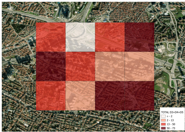
Figure 8. Substantial to heavy damage (D3-D5) were computed up to 35–40% of tall RC buildings due to amplified shaking on soft ground and possible structural irregularities (torsion, weak stories, etc.) in AoI.
